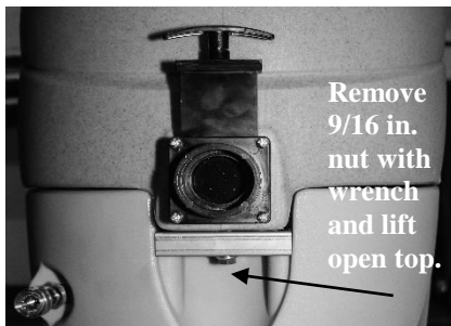
FIG. 4: Solution inlet filter cleaning
