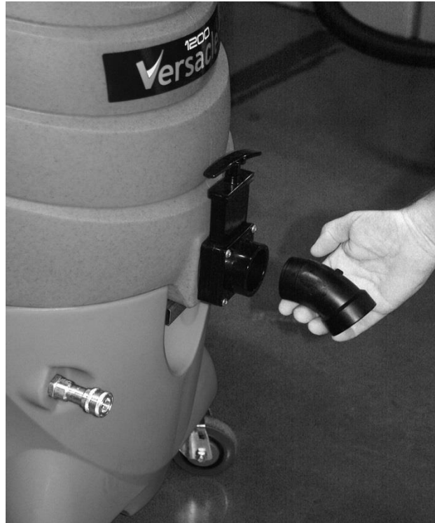
FIG. 7: Gravity drain diverter
